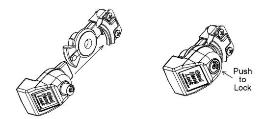
To remove the lock, insert the key into the lock cylinder and turn it clockwise approximately 3/4 turn to release the lock.
