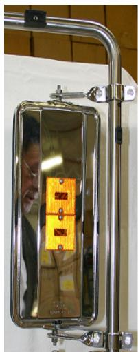
Looking for an alternate mounting solution for your 1 1/8" tubing? Look no further Sure Plus is proud to introduce a Heavy duty twisted mounting bracket to meet your needs. Now you can mount any standard size West Coast mirror on your existing 1 1/8" loop arm. For your spot mirror use the new Heavy duty spot mirror bracket for 1 1/8" tubing. Sure Plus is always looking to meet our customer needs. Order stock now from your local sales representative
